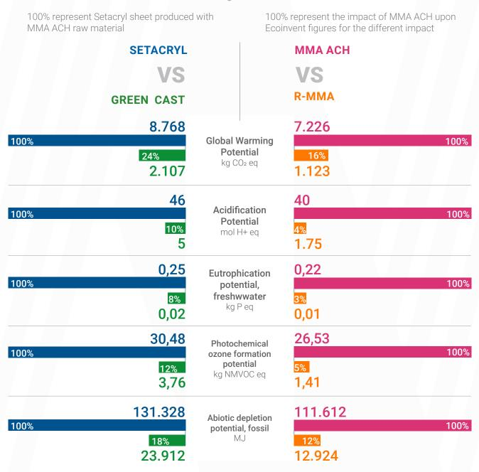
Environmental indicators for impact categories such as Global Warming Potential undergo a considerable decrease of more than 75% compared to a sheet produced with synthetic MMA (ACH).
